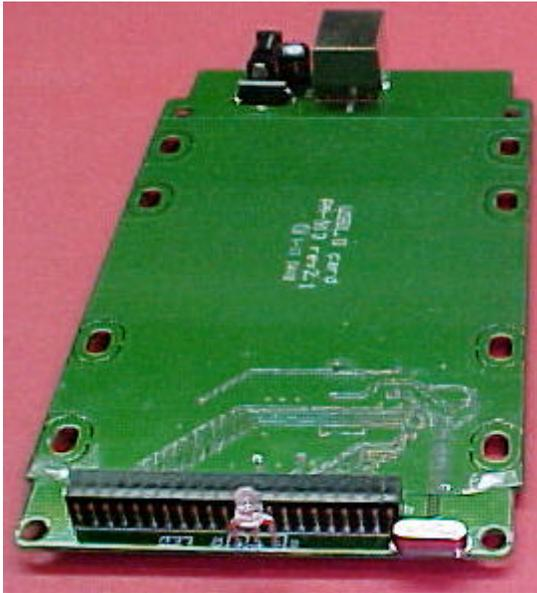
This is your USB external HDD circuit board. When assembled with your disk drive and plugged into the USB port, it will add a drive letter to your computer and allow you to transfer files between your PC and the disk drive.
