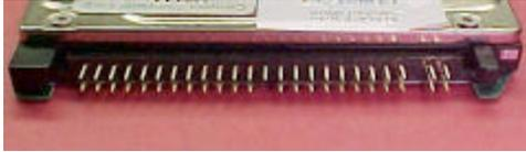
The hard disk drive has two sets of connector pins. 43-pins on the left side and 4-pins on the right.
