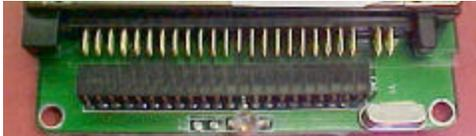
Position the disk drive onto the circuit board then align the left side pins with the connector.
