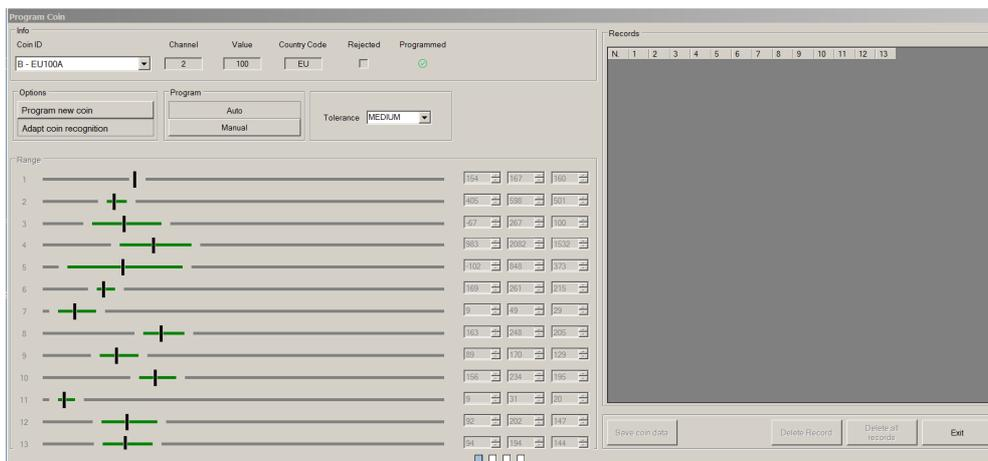
Drop into the acceptor at least 15 pieces. The red data appearing in the monitor screen are the ones read by the sensors. They will be shown in green colour after the 15<sup>th</sup> coin measured.
