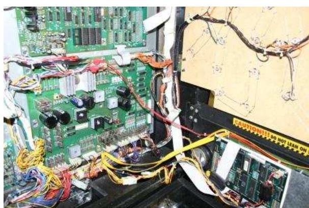
This is the whole setup. **Put the original glass tube power connector aside. The original 8 pin connector of the original display is no longer needed !!!**
