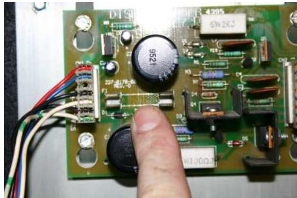
Remove the high voltage fuse on the Display Power Board. That is only for your safety. Otherwise the original display power connector can make a short circuit near the new LED Display.
