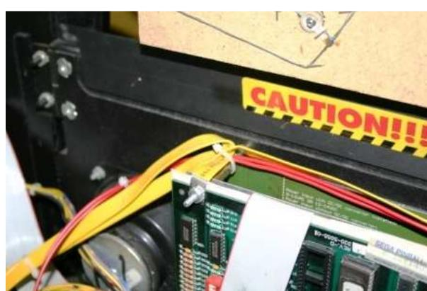
Tighten the ground wires with new cable ties.
