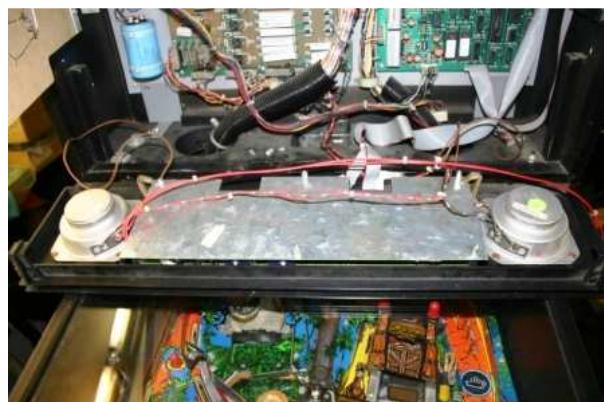
Mount the metal plate back again and tighten the two nuts. Install the four spacers back again.
