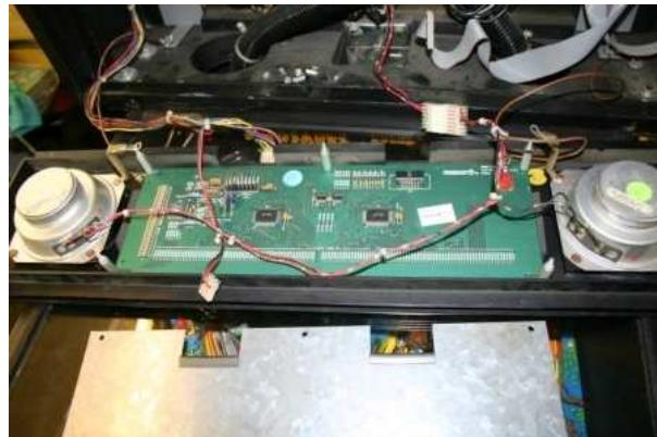
Remove the four spacers of the Display Driver Board. Remove the two left mounting screws and take the metal plate beside.
