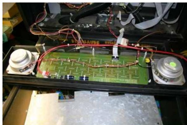
Put the new LED Display in place and mount the five screws again. Connect the flat cable and the in the display set included power supply cable.
