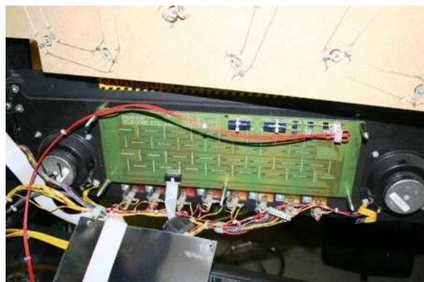
Connect the flat cable and the included power cable to the new display. Install the five washers and the five spacers back again.
