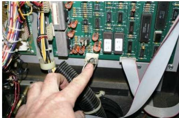
Connect the included display power cable with the two clamps to the two red incoming wires at CN2 pin 2 (black) and pin6 (grey/white).
