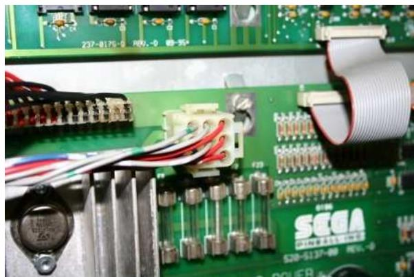
J17 is located on the I/O Power Driver Board. Here you have to connect the included power cable.
