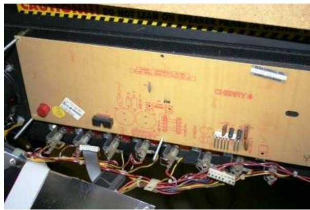
Disconnect the flat cable and the power supply cable from the old display. Remove the five spacers and the five washers from the long mounting screws.
