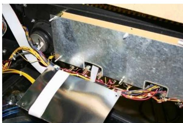
Loosen the four mounting screws of the Display Driver Board and remove it. Remove the three spacers.
