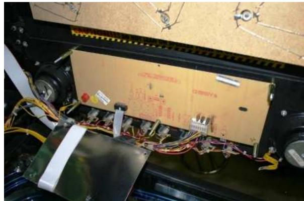
Loosen the two mounting nuts and remove the metal plate.
