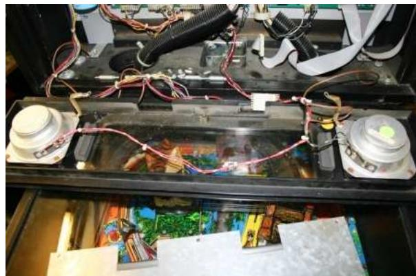
Loosen the five mounting screws of the old display and remove it.
