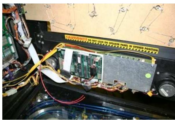
Install the metal plate and the three small spacers from the Display Driver Board back again. Install the Display Driver Board and the ground wires back again.
