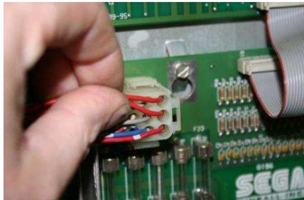
Connect the included red power cable to J17 pin 1 and 4 (both red wires).
